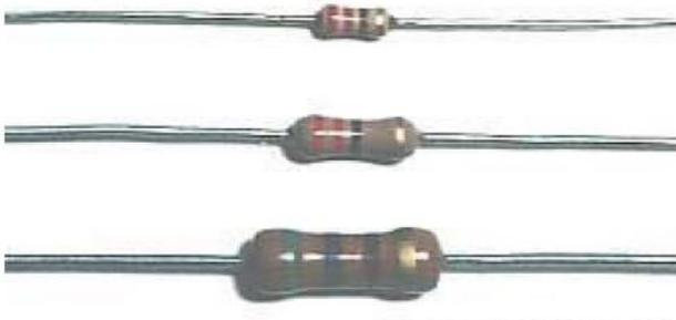
The size of the resistor decides its power rating (i.e., the maximum power it can dissipate without burning).
